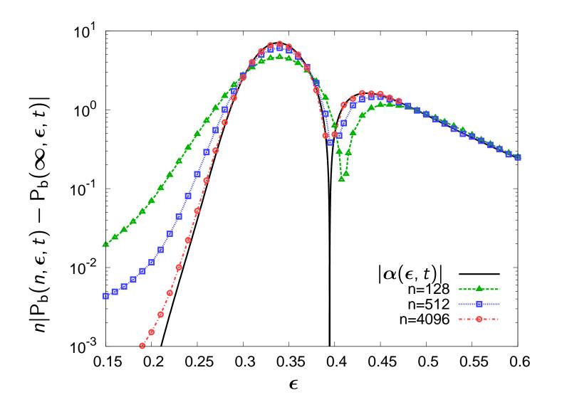
(3, 6)-regular ensemble t=5  $P_b(n, \epsilon, \infty) = \Theta(1/n^2)$  for  $\epsilon < \epsilon_{BP}$  For small  $\epsilon$ , the small number of iteration is sufficient unless blocklength is sufficiently large
